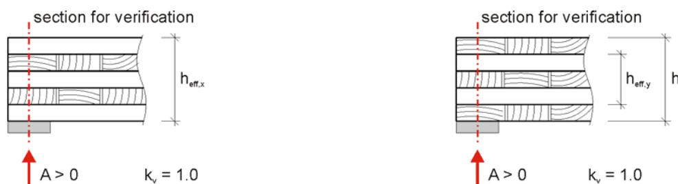
Figure 13: Effective height for calculation of shear stresses
